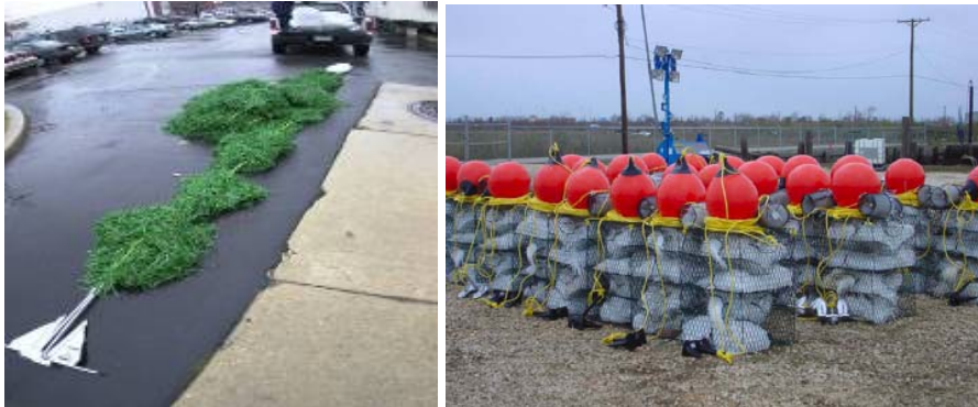
Figure 15. Submerged Oil Recovery System (SORS) and Crab pot oil detectors (Photo credit: NOAA)
