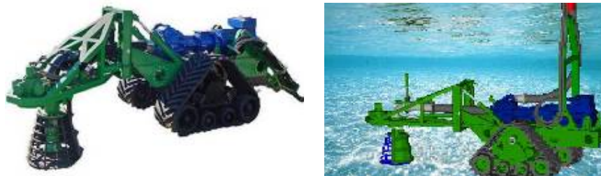
Figure 44 Tornado Motion tracked sunken oil recovery system
