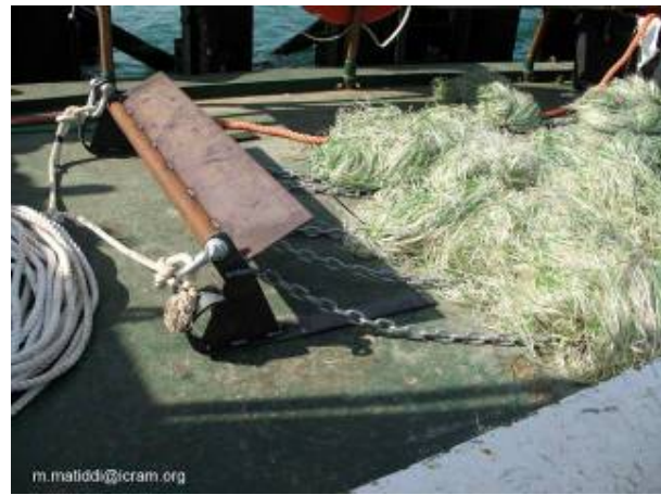
Figure 17. V-SORS used in Falconara oil spill by ISPRA
