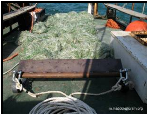
Figure 17. V-SORS used in Falconara oil spill by ISPRA
