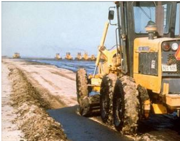
Figure 20. Mechanical Rapid Cleaning To Avoid Oil Remobilisation
