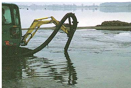
Figure 21. Sunken oil recovery at the Baltic Carrier
