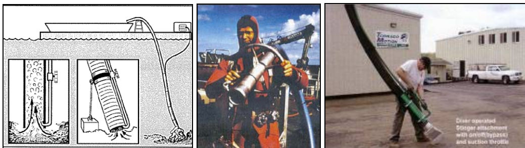
Figure 31. Diver operated suction head or stinger with diver controls (Photo credit HELCOM and Tornado Motion)
