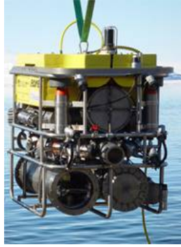
Figure 40 LIDAR system mounted on a R.O.V.
