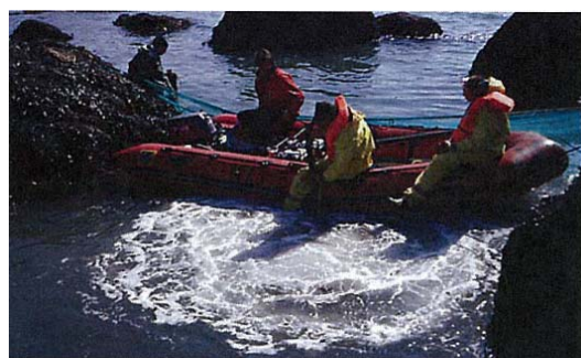
Figure 32. Impact lance used in the Erika incident (photo credit: CEDRE)
